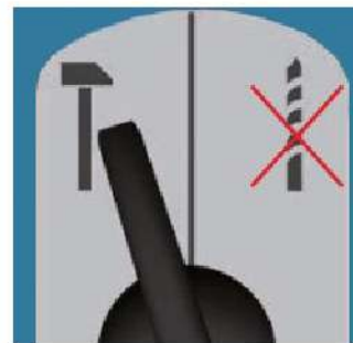
Percussive method for concrete or solid brick substrates.
