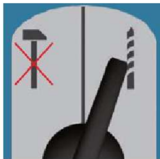
Rotary method for hollow brick substrates
